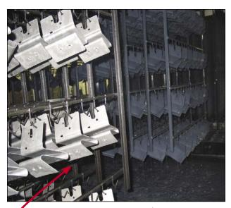
Parts pass through the Burkard electrocoat system. The system is currently being used as a one-color system, but can easily be converted into a two-color system should Burkard wish to add a second color down the road.
