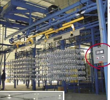
The Programmable Logic Controller (PLC) with racked parts in the background. The control panel is used by operators to enter recipes for various parts and substrates.
