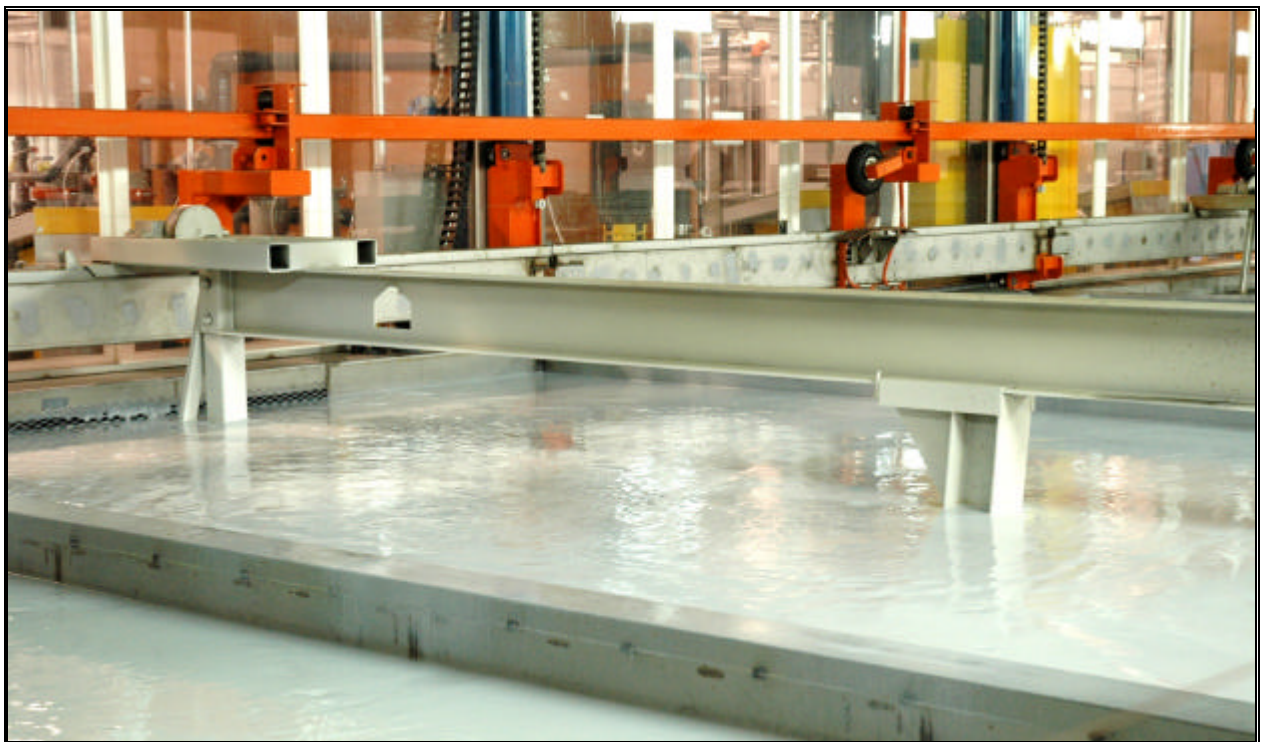
Figure 4. A rocking mechanism tilts truck bodies to assist with air release and drainage.
