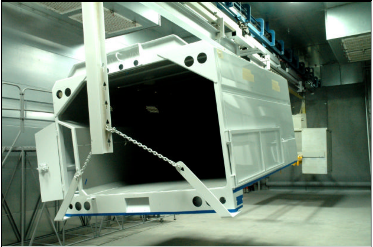
Figure 5. The interiors of these tree care chopper boxes are sprayed with a thick corrosion-resistant coating and do not require electrocoating.
