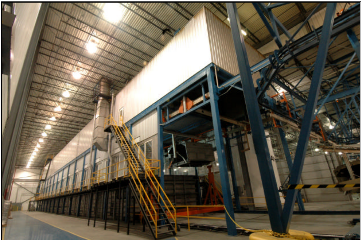
Figure 2. Square transfer electrocoating system at Altec Industries, Burnsville, North Carolina. A tree care truck body is in position to begin the pretreatment process.
