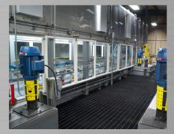
Autodepostion is a water-based, immersion technology that uses chemical reactions to achieve a high quality, uniform finish on the surface of metal. The thickness of the coat depends on submersion time and all exposed surfaces, including tight corners, sharp edges and the insides of tubes and pipes. Due to low curing temperatures, rubber bonded components are not affected. The coating process is typically seven stages or less and bacterial and fungal issues are non-existent.
