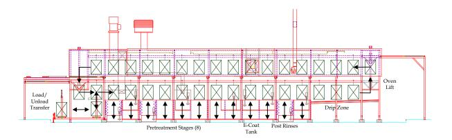
**Figure 1.** Side elevation drawing of square transfer indexing electrocoat system. Part progression is from left to right on lower (process) level and right to left on upper (oven and cool down) level.
