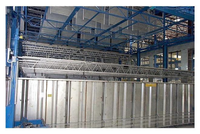
*Figure 3.* In this powder coating system, aluminum parts undergo immersion pretreatment and dryoff in an indexing square transfer system (shown). Loadbars are then transferred to a power and free conveyor for powder application.
