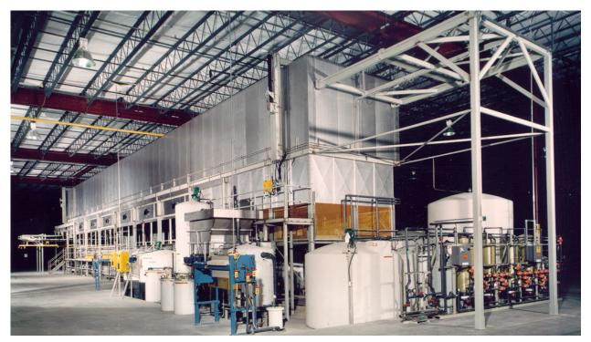
**Figure 2.** Example of an indexing square transfer electrocoat system. Load/unload carousel conveyor is at the far end; cure oven is top, near end; forced cooling zone is top, far end. Water treatment equipment is in the foreground.
