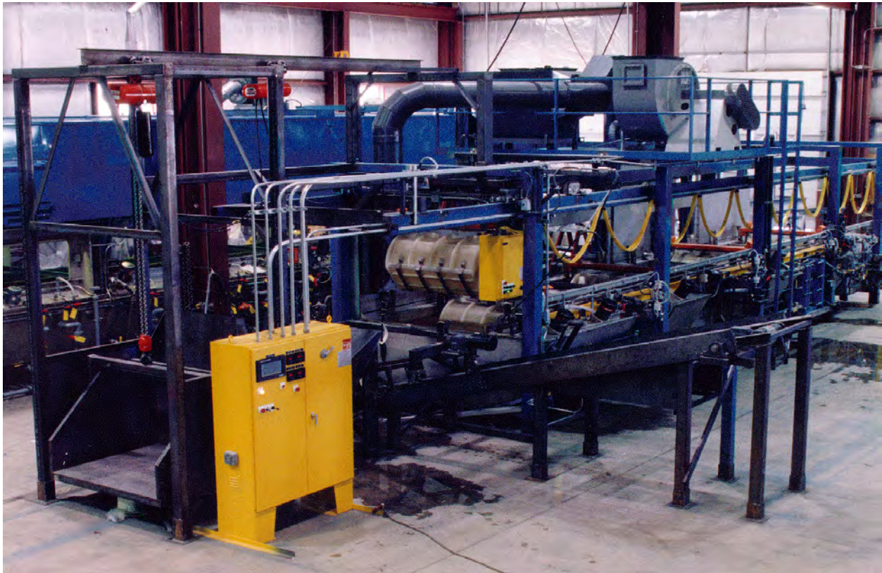
Figure 4. Example of a programmed hoist system. This system has a single, multi-speed traveling hoist for load transfers.
