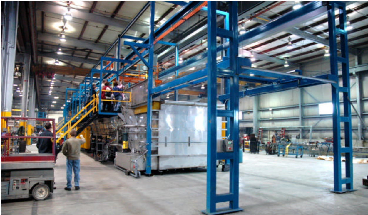
Figure 4. Example of a programmed hoist system. This system has dual variable speed traveling hoists for load transfers.
