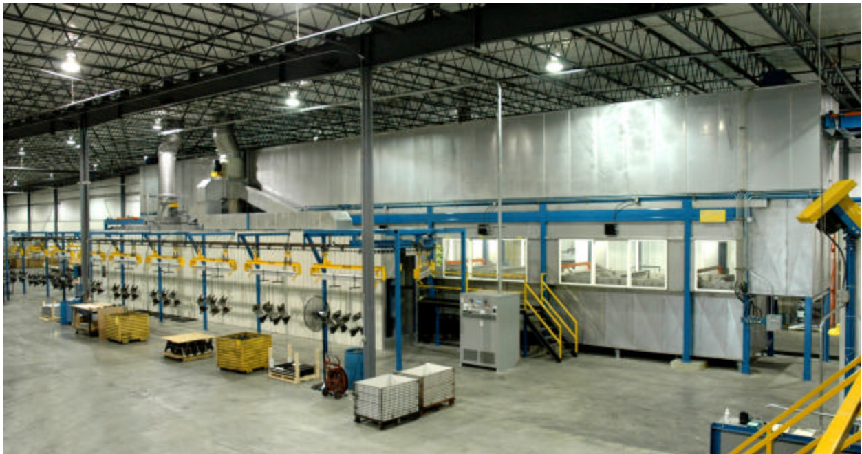
Figure 1. Square transfer indexing electrocoat system. Load/unload carousel conveyor is at left, directly in front of additional forced air cooling tunnel. System photo matches drawing alignment in Figure 2.
